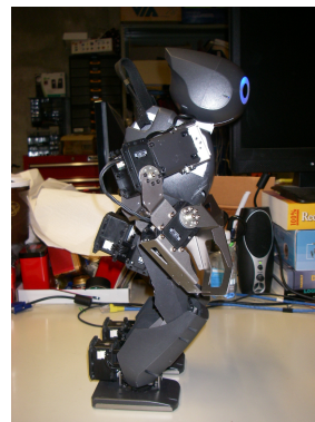
Figure 1: One of our DARwIn-OP robots from the front and side. This robot is equipped with single-DOF hands
