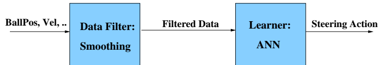
Fig. 3. Level 1: A data filter and a learning technique from level 0 are combined in order to learn a go to point behavior. The input data is first processed by the filter, the passed to the learner which learns a visuo-motor mapping from the input to steering actions.
