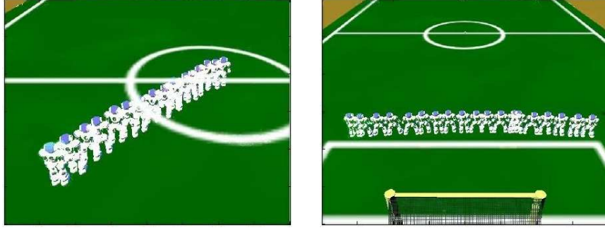
Fig. 2. Two optimized motions in coronal plane: (left) sidewalk, (right) diagonal walk
